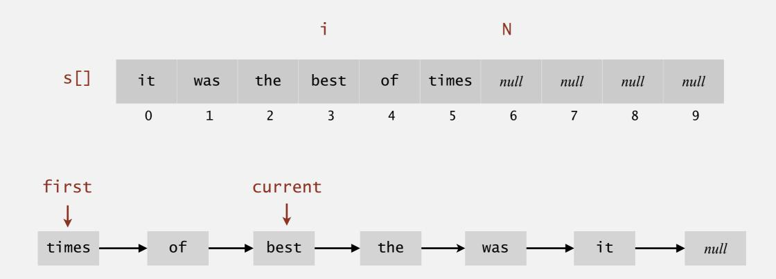
Java solution. Make stack implement the java.lang.Iterable interface.
