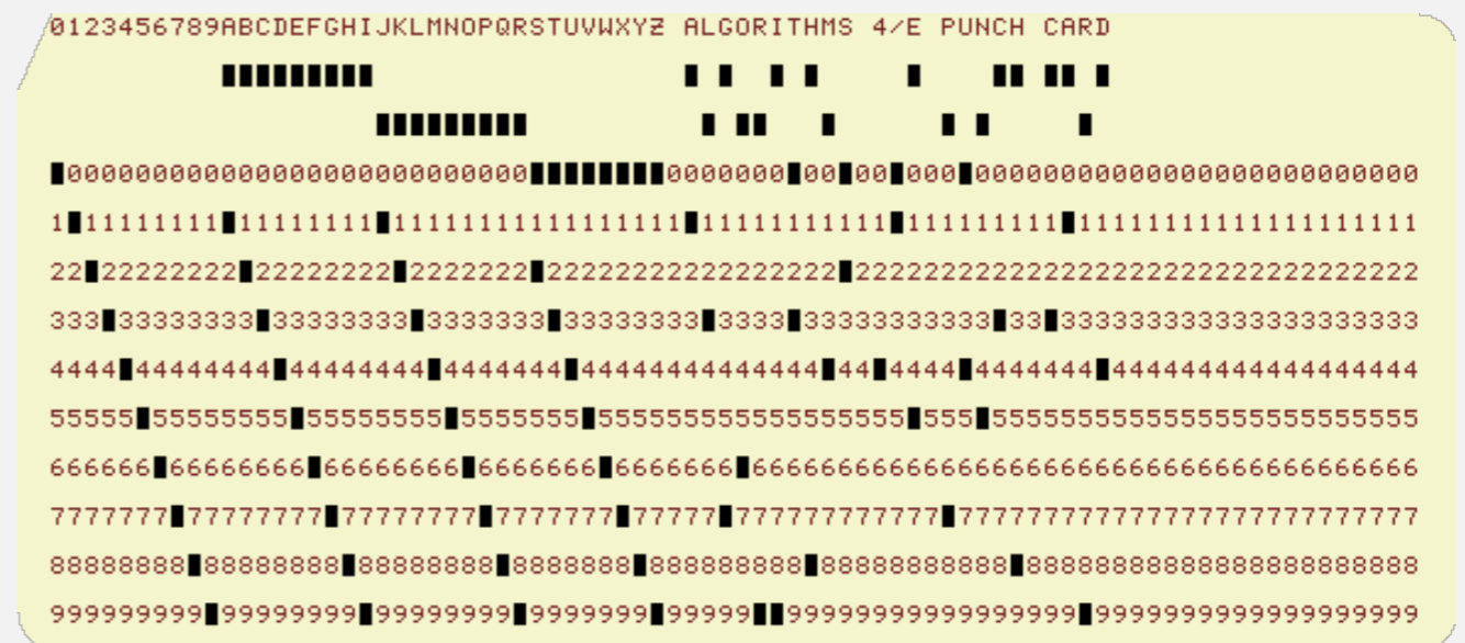
punch card (12 holes per column)
